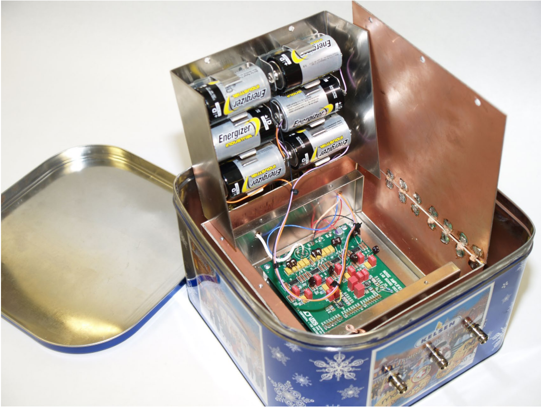
Figure 7. Shielded Box Construction Uses Mu Metal Inside Copper Inside Steel Tin to Attenuate Fields
